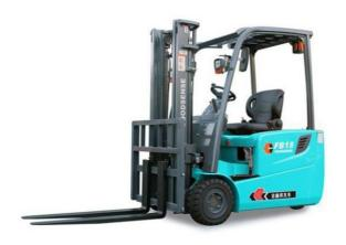
LOOKING FOR A SUITABLE, MULTIPURPOSE FORKLIFT TRUCK WITH EXCELLENT HANDLING? MOBILITY AND TRAFFICABILITY IS CRUX TO THE DESIGN OF GOODSENSE 3 WHEEL ELECTRIC FORKLIFT 2TON, ALLOWING EASY OPERATION IN THE TIGHTEST CONDITIONS. OUR ELECTRIC COUNTERBALANCED TRUCKS ARE AS EFFECTIVE WORKING INSIDE WITHIN PALLET RACKING AISLES AS THEY ARE WORKING OUTSIDE IN THE YARD OR IN A LOADING BAY.
